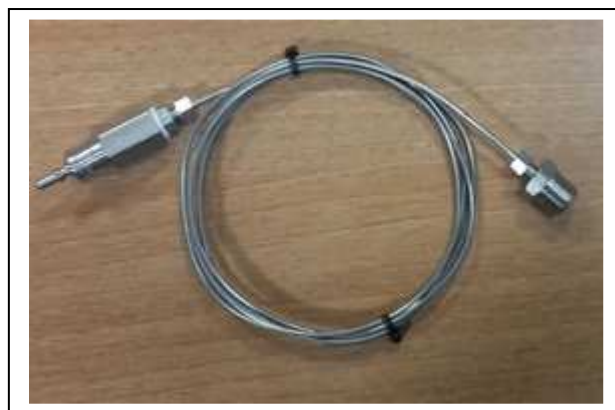
The Hydride Device with the special supplied pipe for the connection to primary H 2 source (H 2 Gas Cylinder or H 2 Generator)
