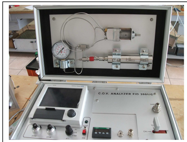
The Hydride Device mounted on the aluminium cover inside the VOC portable monitor
