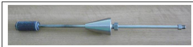
S.S. sampling probe with dust filter on top
